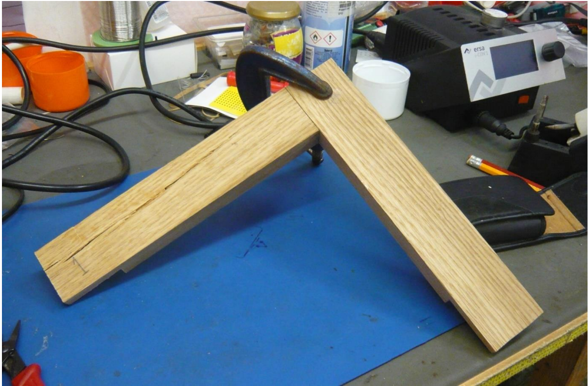
Photo 18: Each of the four joints was glued, using Titebond II wood glue, then held in place with a G-clamp.
