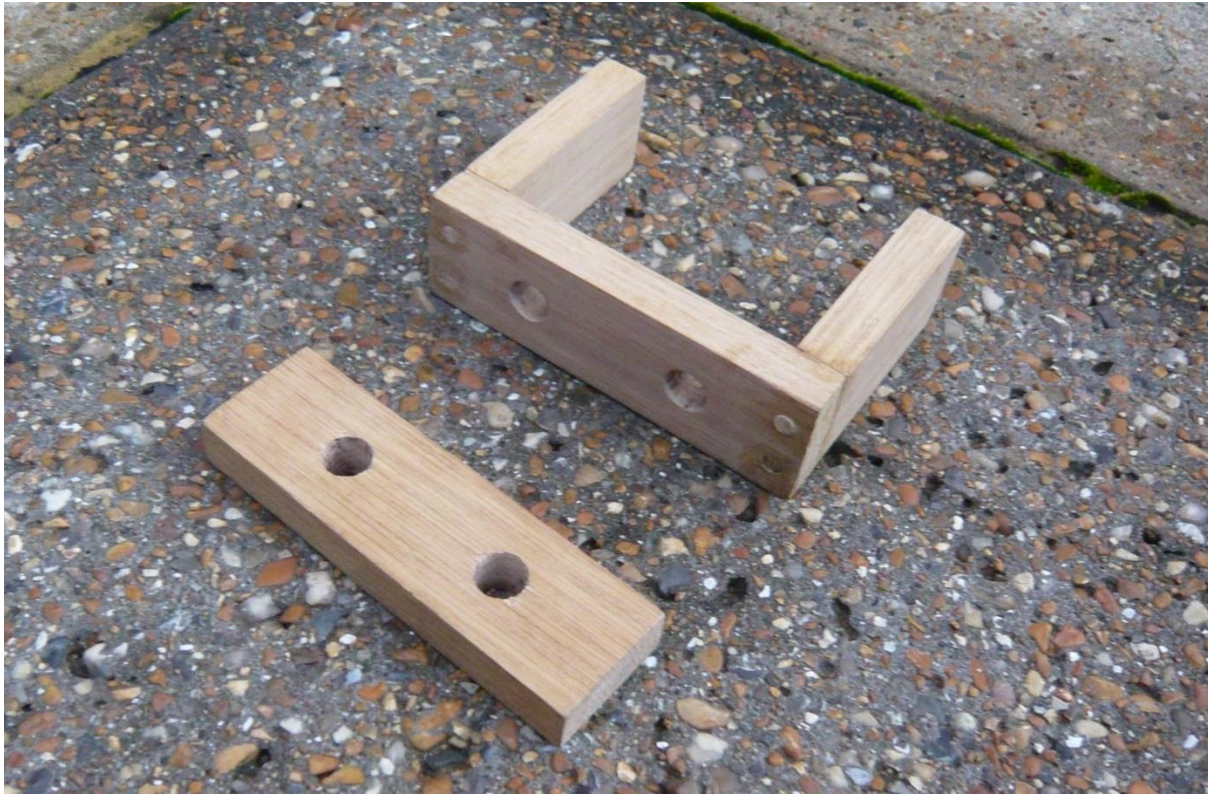
Photo 3: Next, using a smaller piece of oak, I created a second frame using Dowel Joints in each corner.
