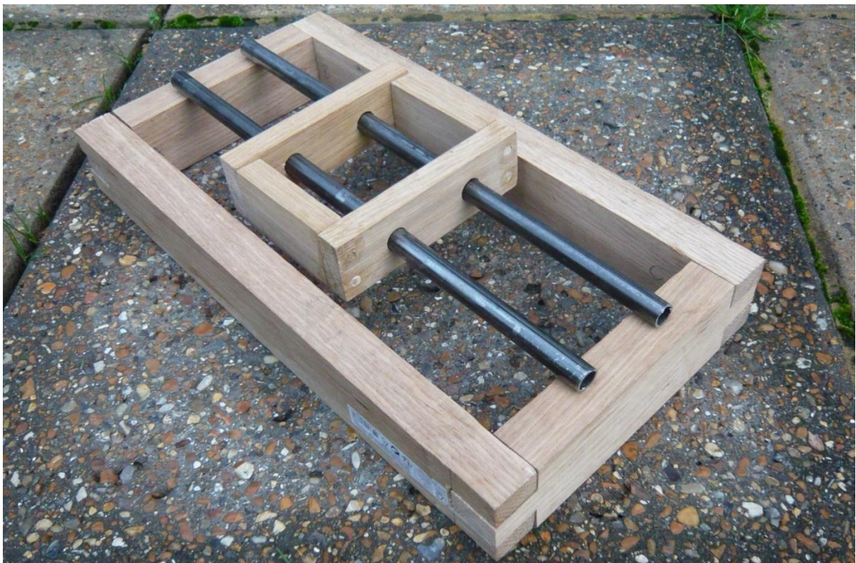
Photo 6: ...shows the fully constructed inner and outer frames of the 'Ball-Bearing Shaft' part of my Drill Press.
