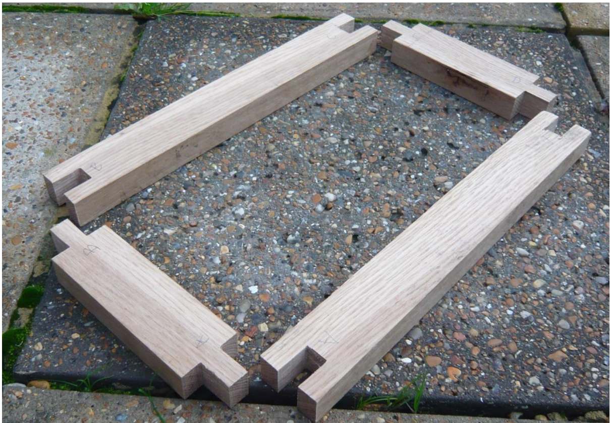
Photo2: Measured out the dimensions for the main frame of my Drill Press. Cut-out 'Box Joints' in each of the four corners using a Band-Saw.
