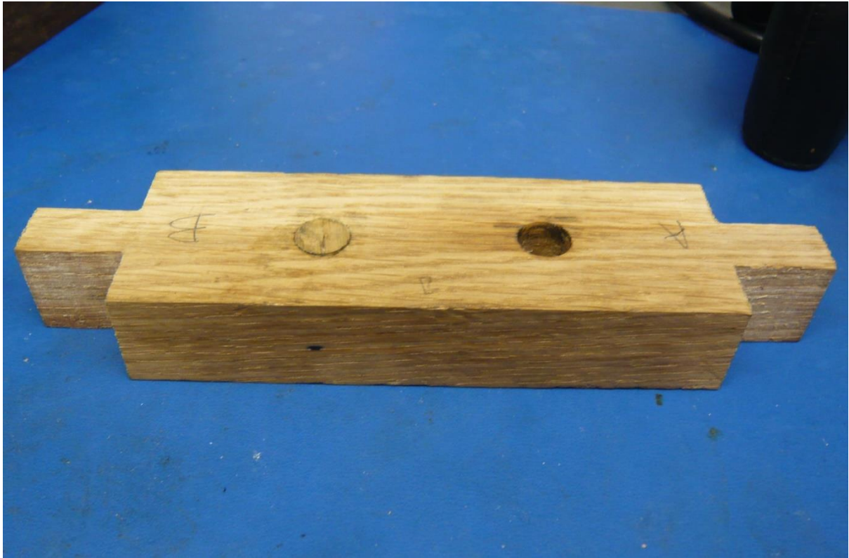
Photo 13: I had to re-drill one of the 12mm holes as the two steel shafts weren't aligned correctly.
