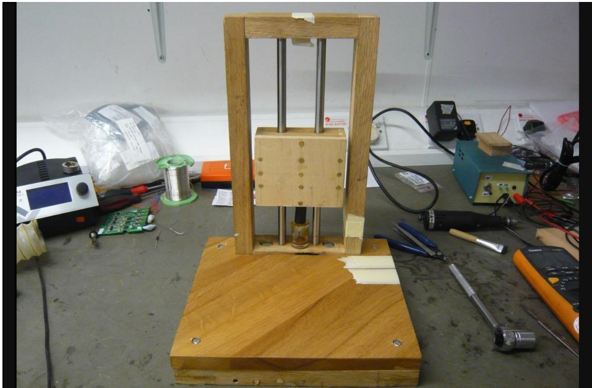
Photo 26: Top view of base showing all bolt heads which have been counter-sunk into the wood.
