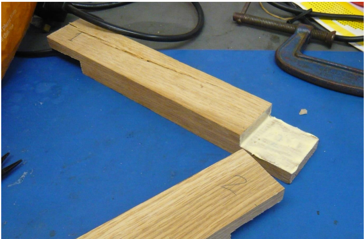
Photo 17: ...same piece of oak used in Photo 1 (Dimensions: 45mm by 25mm by 2500mm). I used 'Half-Lap Joints' for each of the 4 corners.
