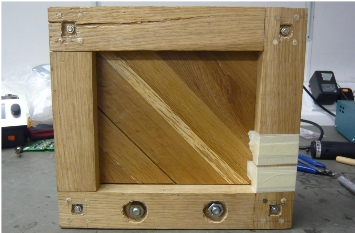
Photo 27: View underneath the base this time showing the six nuts that have been counter-sunk into the wood.
