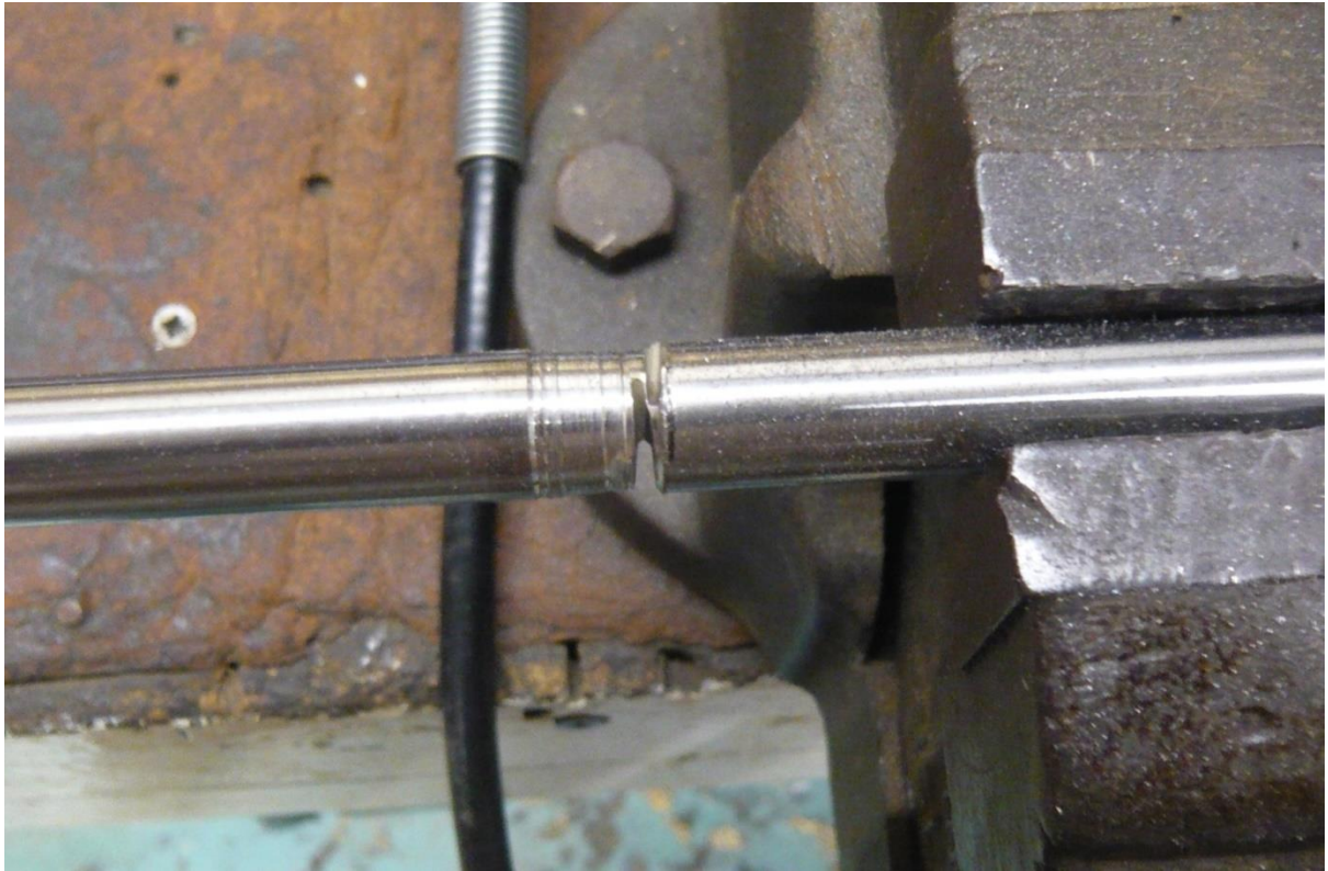
Photo 9: Successfully cutting into steel shaft...
