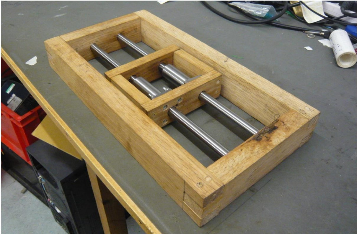
Photo 11: Next, I drilled 4x 12mm holes in the main frame and glued two of its box-joints, using dowel to further strengthen these joints. I left the other two joints unglued so I could extract...
