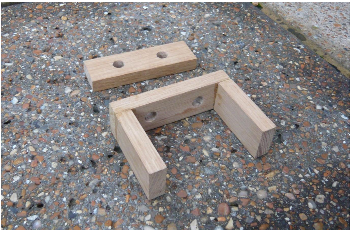
Photo 4: I also drill 2x 12mm holes in both the Top & Bottom Pieces of Oak. These were for two Steel Shafts to be slotted through.
