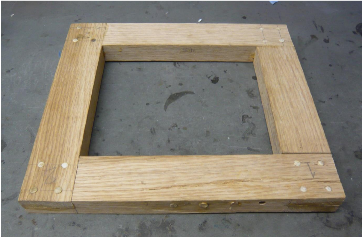
Photo 22: Completed base frame with dowel inserts.
