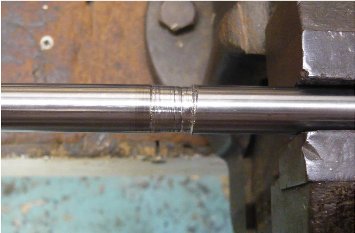
Photo 7: I purchased a piece of hardened-steel shaft (12mm diameter by 600mm) from Bearing Boys ( www.bearingboys.co.uk ), which I planned to chop in half so creating two separate shafts.
