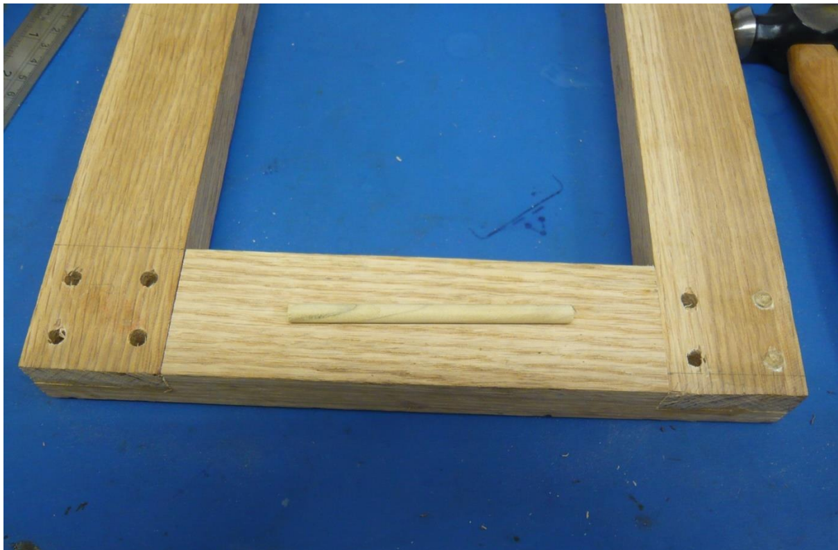
Photo 21: For each of the four corners I then drilled 4x 6mm holes, fully through the wood, then inserted 6mm dowel (with glue) in each hole to add extra strength.
